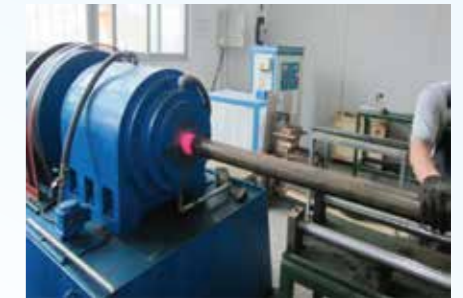
Making the pointed head of the pipe
